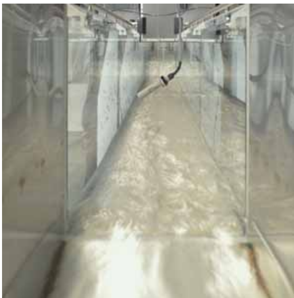
FLOAT SWITCH IN CHANNEL
