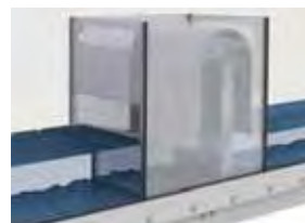
SIPHON SPILLWAY (FC300L)
