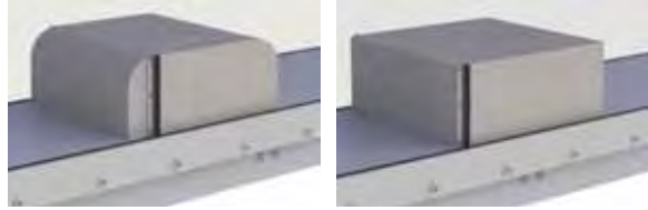
PAIR OF BROAD CRESTED WEIRS (FC300R): STREAMLINED (LEFT), SHARP CORNERED (RIGHT)
