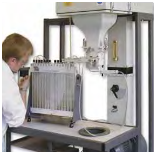
SHOWN FITTED WITH ONE OF THE AVAILABLE EXPERIMENT MODULES (AF12) AND MULTI-TUBE MANOMETER (AF10A)
