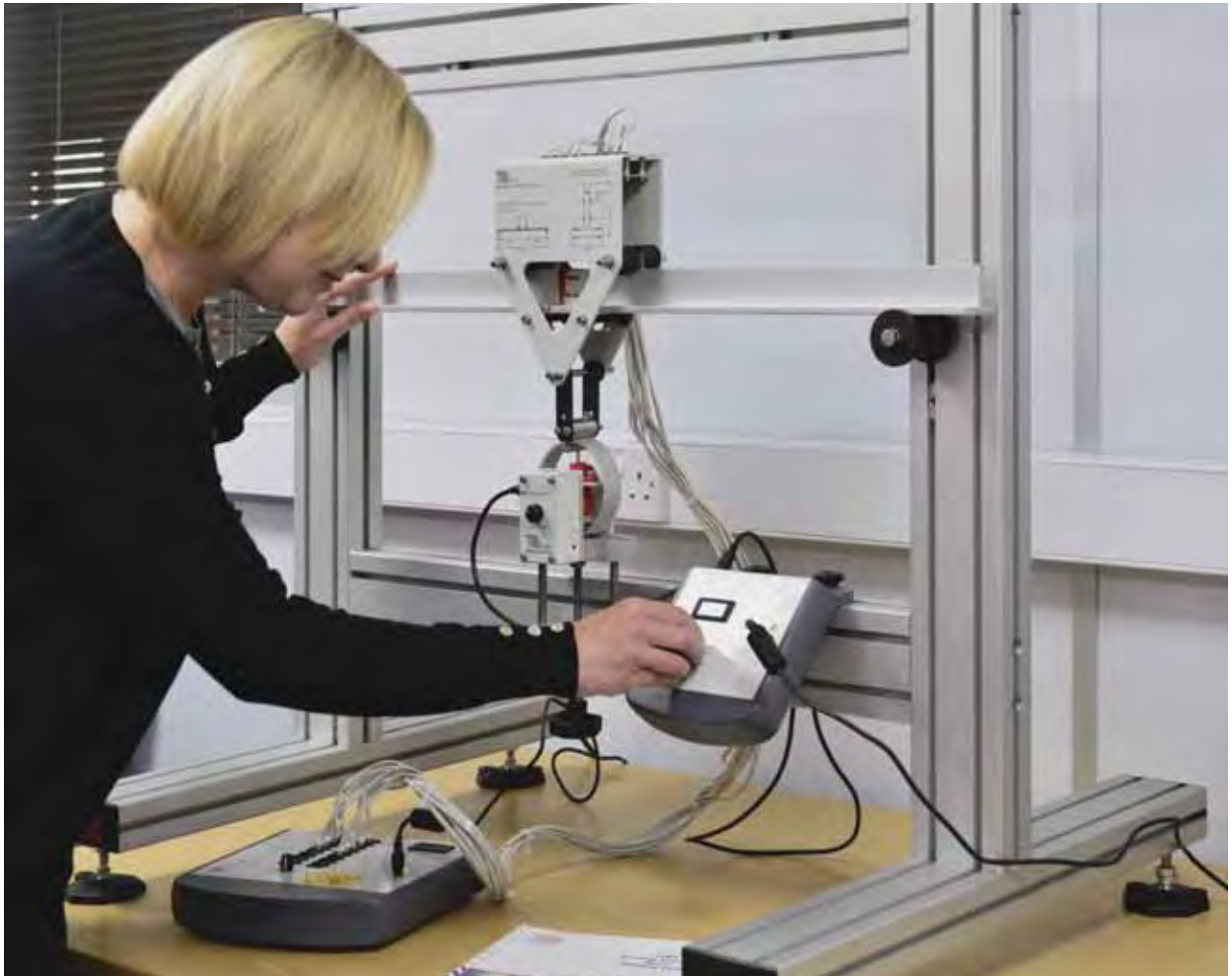
TEST FRAME (STRI) FITTED WITH THE EXPERIMENT MODULE BENDING STRESS IN A BEAM (STR5) AND DIGITAL FORCE DISPLAY (STRIA)
