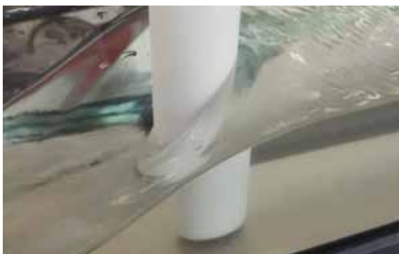
SUBCRITICAL AND CRITICAL FLOW PAST PIER
